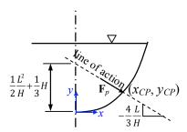
In order to find  $(x_{CP}, y_{CP})$ , we would need to find the intersection of the line of action with the equation of the wall (Eq. (2.44)). This calculation is tedious for the current example and will not be performed here.
