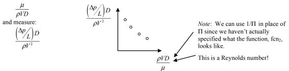
All of the information contained in the previous four plots is contained within this single plot! This reduces the complexity, cost, and time required to determine the relationship between the average pressure gradient and the other variables.
