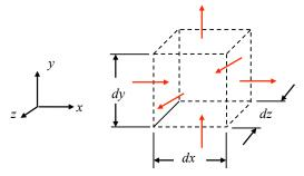
Assume that the density and velocity are  $\rho$  and  $\mathbf{u}$ , respectively, at the control volume's center. The mass fluxes through each of the side of the control volume are given by:
