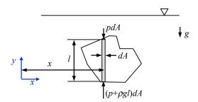
$$x_{CB}\hat{\mathbf{i}} \times \underbrace{\rho g V \hat{\mathbf{j}}}_{\text{buoyant force}} = \int_{A} x \hat{\mathbf{i}} \times \underbrace{\rho g l d A \hat{\mathbf{j}}}_{\text{net pressure force on parrow collinder}}$$
