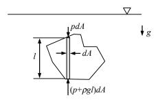
The net pressure force in the vertical direction on the narrow cylinder, assuming an incompressible fluid, is,
