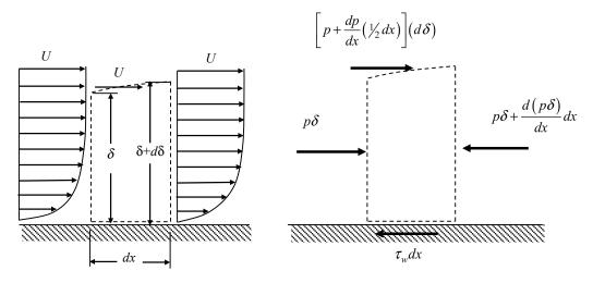
Let's apply the linear momentum equation in the *x*-direction to the control volume:
