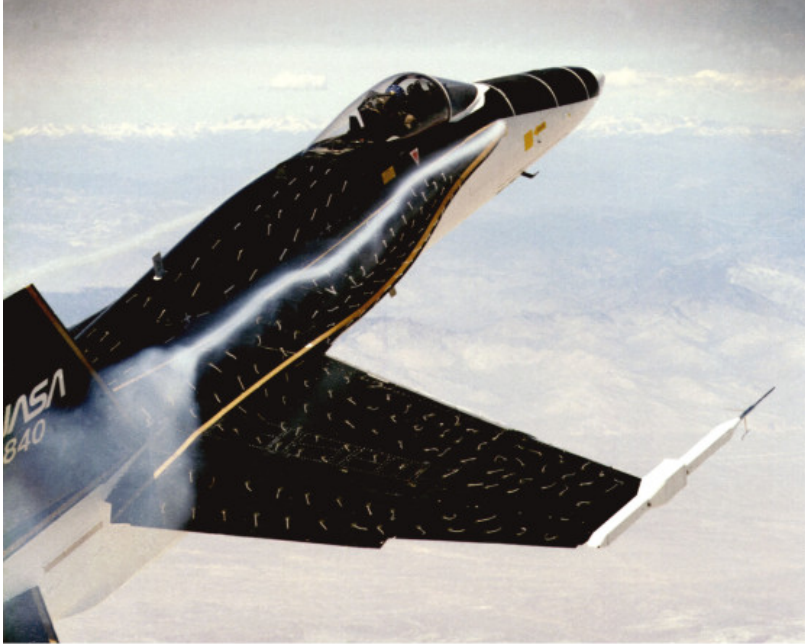
Dryden Flight Research Center EC89-0096-206 Photographed 1989 F-18 HARV smoke and tuft flow visualization. Angle of Attack = 20 deg. NASA photo.
