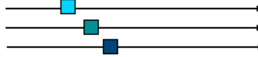
FIGURE 5.5. The density of fluid particles varies from layer to layer in this stratified flow, but remains constant within a layer.
