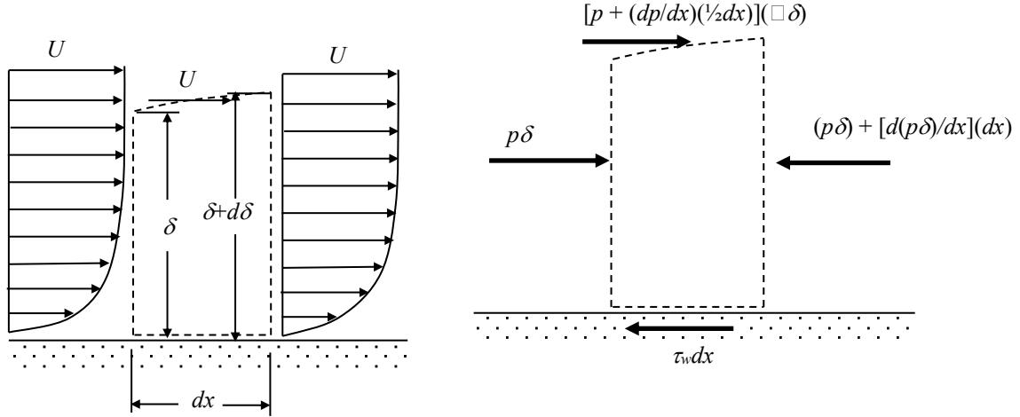
$$\underbrace{-\dot{m}_{\text{top}}}_{\text{in through top}} - \underbrace{\int_0^\delta \rho u dy}_{\text{in at left}} + \underbrace{\left[ \int_0^\delta \rho u dy + \frac{d}{dx} \left( \int_0^\delta \rho u dy \right) dx \right]}_{\text{out through right}} = 0$$
