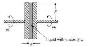
Develop an expression for the torque, T, transmitted by the disk pair, in terms of the liquid dynamic viscosity,  $\mu$ , the disk radius, R, the disk spacing, a, and the angular speeds of the input disk,  $\omega$ , and output disk,  $\omega$ .
