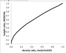
An alternate approach for deriving Eq. (17) is to sum moments about the hinge, but make note of the fact that the center of pressure on each wall is one-third of the liquid depth from the bottom of the wall,
