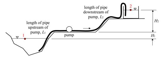
$$\left(\frac{p}{\rho g} + \alpha \frac{\overline{V}^2}{2g} + z\right)_2 = \left(\frac{p}{\rho g} + \alpha \frac{\overline{V}^2}{2g} + z\right)_1 - H_L + H_S , \qquad (1)$$
