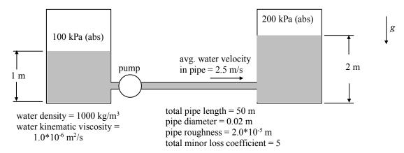
Determine the power the pump must provide to the water to maintain the given conditions.
