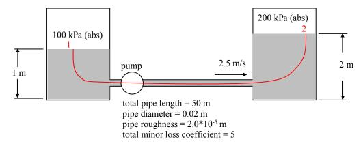
$$\left(\frac{p}{\rho g} + \alpha \frac{\overline{V}^2}{2g} + z\right)_2 = \left(\frac{p}{\rho g} + \alpha \frac{\overline{V}^2}{2g} + z\right)_1 - H_L + H_S \tag{1}$$
