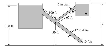
In the water flow system shown, reservoir B has variable elevation, x. Determine the water level in reservoir B so that no water flows into or out of that reservoir. The speed in the 12 in diameter pipe is 10 ft/sec. Assume the pipes are constructed of cast iron and that the entrances are sharp-edged.
