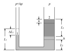
$$\underbrace{\rho_{2}}_{=p} = \underbrace{\rho_{1}}_{=p+\Delta p} + \rho_{H20}g(L_{1} - \Delta L_{1}) - \rho_{H20}g(L_{2} + h) - \rho_{Hg}gL_{3}
