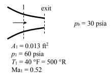
First determine whether or not the flow is choked by checking the pressure ratio at the exit. In order to do this, we must first determine the flow stagnation pressure (we'll also calculate the stagnation pressure while we're at it). Note that the flow remains subsonic in the nozzle (subsonic Mach number and no minimum area) so that there will be no shock waves in the flow to modify the flow's stagnation pressure.
