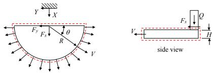
$$\frac{d}{dt} \int_{CV} u_X \rho dV + \int_{CS} u_X \left( \rho \mathbf{u}_{\text{rel}} \cdot d\mathbf{A} \right) = F_{B,X} + F_{S,X}$$
