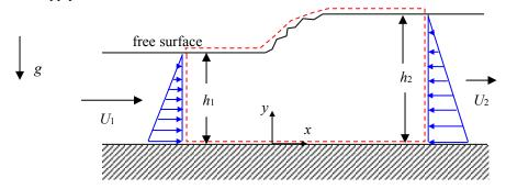
Note: Since the streamlines are parallel at the inlet and outlet of the CV, the pressure gradient normal to the streamlines will be hydrostatic.
