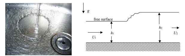
The depth increases suddenly from  $h_1$  to  $h_2$  downstream of the jump. The jump itself is often turbulent and involves viscous losses so that the total pressure downstream is less than that of the upstream flow.
