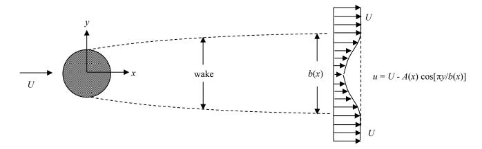
The surveys are made at x locations sufficiently far downstream of the body so that the pressure across the wake is the same as the ambient pressure in the fluid far from the body. The surveys indicate that, to a first approximation, the velocity in the wake varies with lateral position, y, according to:
