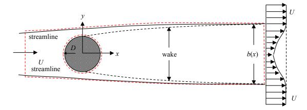
$$\frac{d}{dt} \int_{\text{CV}} u_x \rho dV + \int_{\text{CS}} u_x \left( \rho \mathbf{u}_{\text{rel}} \cdot d\mathbf{A} \right) = F_{B,x} + F_{S,x} \tag{1}$$
