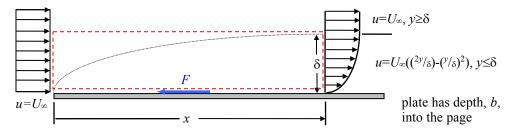
Determine the mass flow rate out of the control volume through the top using conservation of mass.
