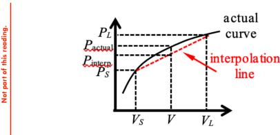
FIGURE 3.24. Schematic showing how to linearly interpolate a property value.
