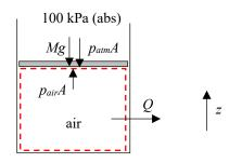
Apply the First Law of Thermodynamics to a system consisting of the air inside the piston (indicated by the red, dashed line in the figure),
