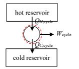
(Note  $Q_C < 0$  since heat leaves the system. We're also assuming that the temperature at the boundaries to the system where the heat is added/removes is the same as the adjacent reservoir.) Thus, we see that the cycle is internally reversible.
