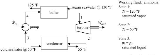
isentropic turbine efficiency = 0.80isentropic pump efficiency = 0.85
