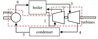
$$\frac{dE_{CV}}{dt} = \dot{Q}_{into\ CV} - \dot{W}_{by\ CV} + \sum_{in} \dot{m} \left( h + \frac{1}{2}V^2 + gz \right) - \sum_{out} \dot{m} \left( h + \frac{1}{2}V^2 + gz \right), \tag{2}$$
