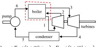
$$\frac{dE_{CV}}{dt} = \dot{Q}_{into\ CV} - \dot{W}_{by\ CV} + \sum_{in} \dot{m} \left( h + \frac{1}{2} V^2 + gz \right) - \sum_{out} \dot{m} \left( h + \frac{1}{2} V^2 + gz \right), \tag{8}$$
