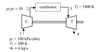
Calculate the thermal efficiency for the Brayton cycle,
