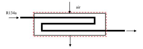
$$\frac{dE_{CV}}{dt} = \sum_{in} \dot{m} \left( h + \frac{1}{2} V^2 + gz \right) - \sum_{out} \dot{m} \left( h + \frac{1}{2} V^2 + gz \right) + \dot{Q}_{added \ to \ CV} - \dot{W}_{by \ CV, other},\tag{5}$$
