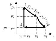
To find the work and heat transfer, apply the 1<sup>st</sup> Law to every process and make use of the ideal gas relations.
