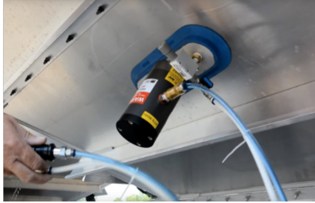
FIGURE 11.16. A wall vibrator attached to a hopper wall. This figure is from http://www.shake-it.com/product-line/mt-fast-hopper-trailer-vibrator/ .
