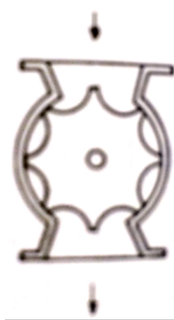
FIGURE 11.13. Illustration of a rotary valve with shallow pockets, which can be used to decrease the flow rate. This figure is from Thomson [5].
