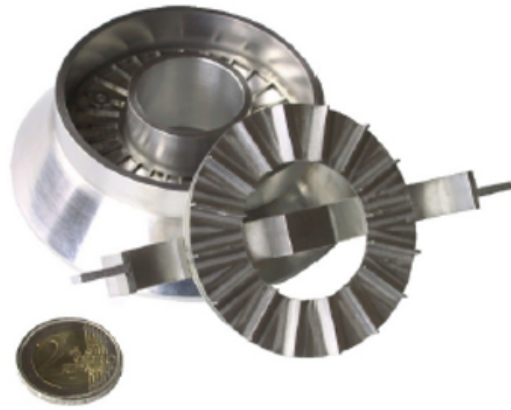
Shear cell approx. 30 ml, 2 EURO coin
