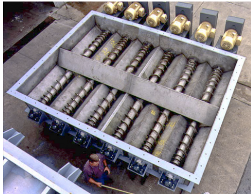
FIGURE 11.5. A photograph of a “live bottom” screw feeder to be located at the bottom of a hopper with a large exit area. This photograph is from http://www.conveyoreng.com/products/screw-feeders-live-bottoms/?v=868f8823ca02 .
