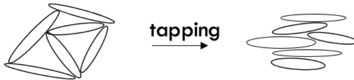
FIGURE 2.5. (left) Powders gently poured into a container can support large void spaces if the particles are frictional or cohesive, resulting in a small bulk density. (right) After tapping, these voids collapse and the bulk density increases.
