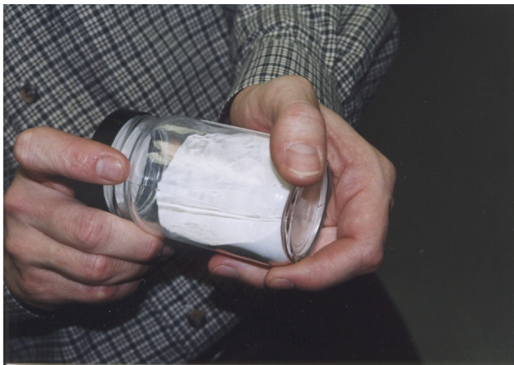
FIGURE 2.1. The traditional assessment of powder flowability consists of an experienced worker tumbling a jar of powder and, based on that person’s experience, assessing the powder’s “flowability”. This photograph is courtesy of B. Hancock.
