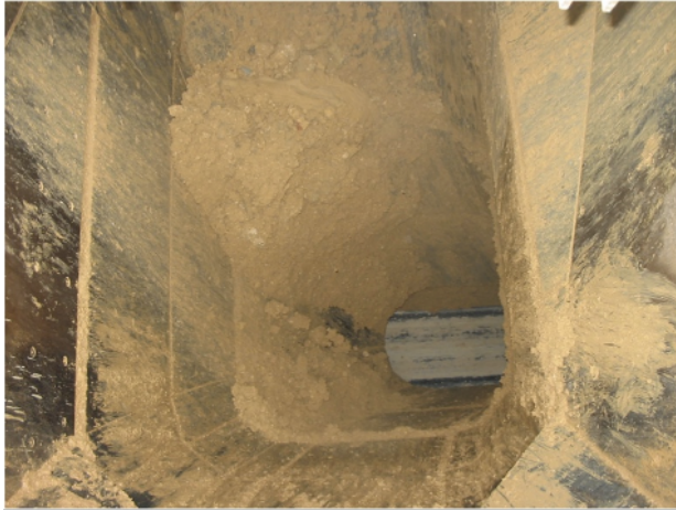
(A) Photo showing build-up of material in a chute.
