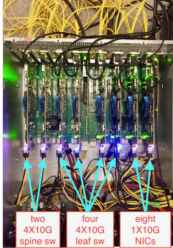
Figure 1.10: Small-scale network for evaluation comprising 8 end-host NICs and 6 switches connected in a two-tier Fattree topology with full bisection bandwidth (also known as leaf-spine topology) connected inside the PCIe expansion system.
