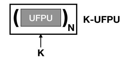
K-UFPU comprises N UFPUs and adds a new configurable parameter K
