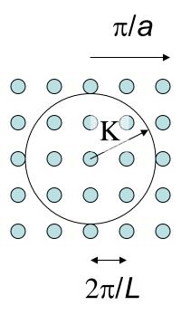
$$D(\omega) = \frac{1}{L^{\alpha=2}} \frac{dN}{d\omega} = \frac{1}{V} \frac{dN}{dK} \frac{dK}{d\omega} = \frac{K(\omega)}{2\pi} \frac{1}{v_g(\omega)}$$
