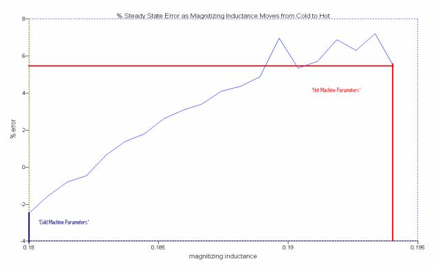
'Crunchiness' is due to torque ripple, stability at higher Lm
