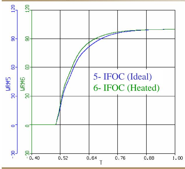
• Error in controller parameters produce a difference in speed of the machine
