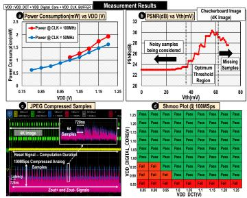
Fig. 5.(a) Power consumption vs VDD at 50MHz and 100MHz. (b) PSNR variation vs ADC threshold voltage (c) Measurement waveforms showing compressed analog samples, zoomed in set of 64 analog samples for a 8x8 matrix (d) Shmoo Plot.
