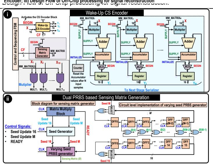
i) Architecture of the proposed Wake-up CS Encoder, presenting the associated control signals and the power-gating to reduce the overall power consumption; ii) Control flow and Circuit Diagram of the Dual PRBS sensing matrix sensing matrix generation.
