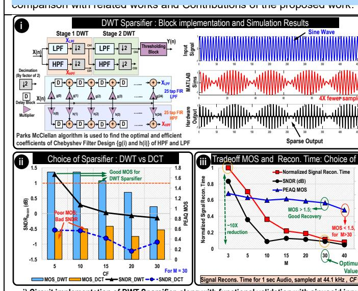
i) Circuit implementation of DWT Sparsifier, along with functional validation with sinusoid input; ii) Benefits of DWT over DCT in terms of MOS and SNDR; iii) Design choice of value of M in the CS Encoding, showing the trade-off between signal reconstruction time and MOS
