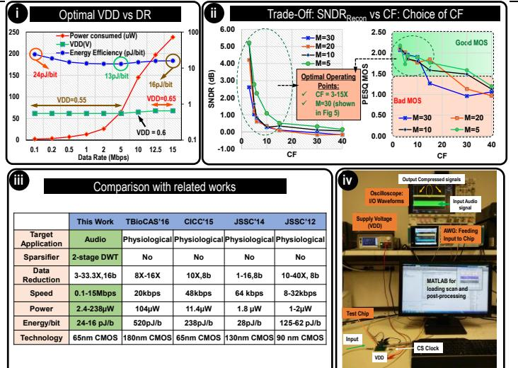
i) Optimal supply voltages for different DR to achieve lowest operating energy efficiency; ii) Choice of CF for effective reconstruction of audio signal; iii) Performance comparison of implemented CS IC with state-of-the-art CS Encoders; iv) Measurement Setup
