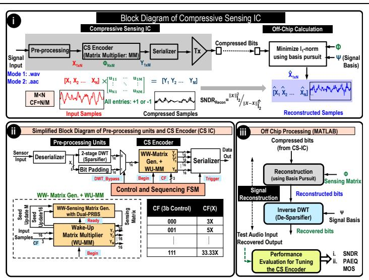
i) System-level block diagram of the implemented CS, depicting the On-chip CS Encoder and Off-Chip Reconstruction; ii) Architecture of CS Block, utilizing the 2-stage DWT Sparsifier and Wake-Up Encoder; iii) Design Flow of Off-Chip processing for signal reconstruction.
