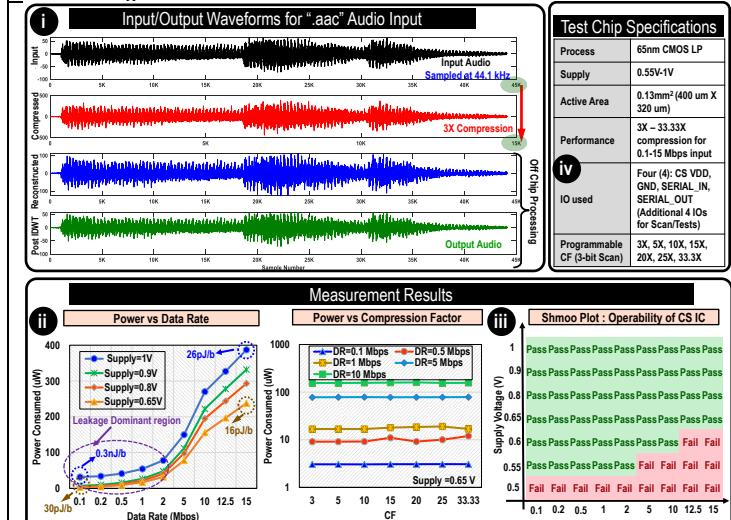
Measurement Results for CS IC: (i) Input-Output Timing diagram for Audio Input, ii) Variation of power with input Data Rate and Compression factor, iii) Shmoo plot, depicting the operability of the IC at different DR and Supply voltages, iv) Chip Specifications
