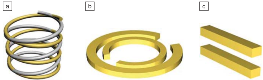
Figure 1. (a) Schematic of a bihelix structure. The gold helix is left-handed, and the silver helix is right-handed. The two helices are shown in different colors to improve clarity. In a real device, both helices are made using the same material. (b) Schematic of a pair of split-ring resonators. In the case of a single split-ring resonator, the inner resonator is missing. (c) Schematic of a pair of nanorods.
