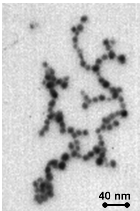
Figure 1. A transmission electron microscope (TEM) picture of the silver aggregate used in the experiments.
