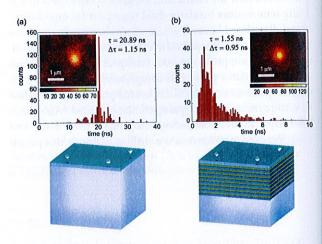
Figure 2: Experimentally measured spontaneous emission lifetimes. Histograms of the NV center lifetimes on (a) coverslip and (b) HMM. Corresponding mean values (standard deviations) of the lifetime distributions are: (a) 20.89 ns (1.15 ns), (b) 1.55 ns (0.95 ns).
