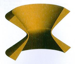
Figure 1: Unbound iso-frequency surfaces for  $\omega$  and  $\omega + \delta \omega$  that define the anomalously large photonic density of states in a hyperbolic metamaterial (HMM).
