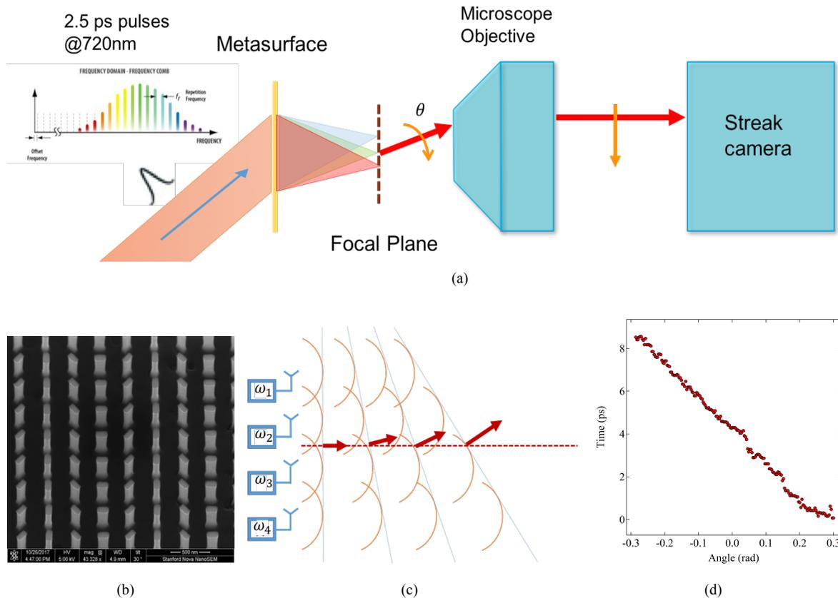
Figure 1: (a) Schematics of experimental Setup consisting of a frequency-comb source (picosecond pulse), silicon-based metasurface, microscope objective and streak camera. (b) SEM image of a section of the fabricated Silicon based metasurface. (c) Conceptual schematic of beam steering using frequency-arrayed source. (d) Experimental measurement of the streak camera showing the beam steering action.
