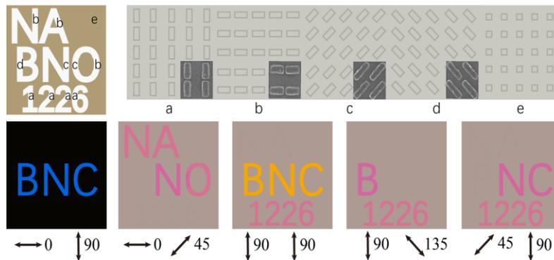
Fig. 2. Highly secure information encryption. Different building blocks (indicated by a-d) are generated by rotating the nanoantenna with a step of 45°. Squared nanoparticles are used as the background of the layout (e). The insets show the scanning electron microscope images of fabricated antennas. The bottom row shows calculated images decrypted by 5 different combinations of polarization states from the same layout shown in top left image.
