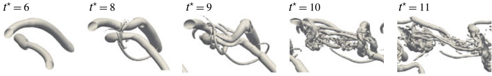
FIGURE 12. Description of the orthogonal reconnection event occurring for the case h/R=0.61 , r_c/h=0.166 and Re_\Gamma=7000 . Q -criterion iso-surfaces plotted in the region of interest at different times during the reconnection.
