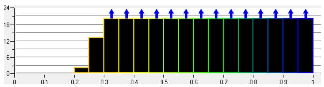
Figure 178: Quality Histogram for Tetra/Prism Mesh after Smoothing
