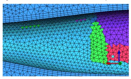
Figure 197: Zoomed-in Mesh—Slivers Meshed with Equilateral Triangles
