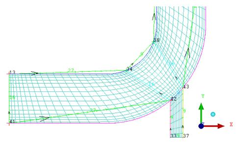
Figure 18: Mesh After Matching Edges
