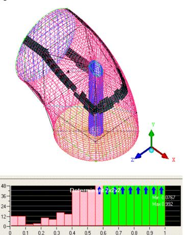
Figure 125: Skewed Cells (Below 0.6) in the Pre-Mesh
