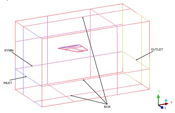
Figure 171: Part names for External Surfaces
