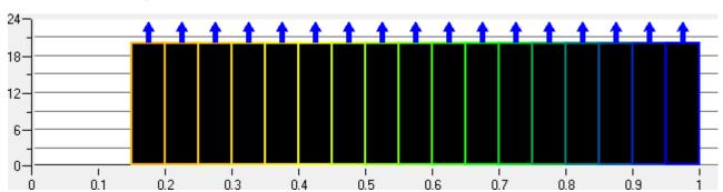
Figure 180: Quality histogram for Hexa-Core mesh
