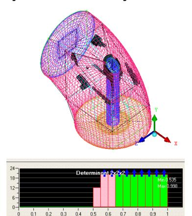
Figure 138: Worst Cells After Adding Cells
