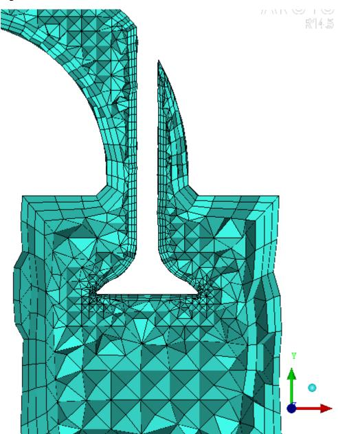
Figure 189: Tetra/Prism Volume Mesh around Valve
