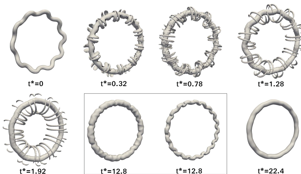
Figure 2. The Q -criterion contours (The threshold is set to yield the best visualization at Q\Gamma^4 R^{-6}=1907 ) of Case A-I for various times corresponding to the evolution of the vortex ring with initial perturbation. Plots of t^* = 12.8 in box are generated with different Q iso-surfaces ( left : Q\Gamma^4 R^{-6}=1907 ,right: Q\Gamma^4 R^{-6}=3814 ).
