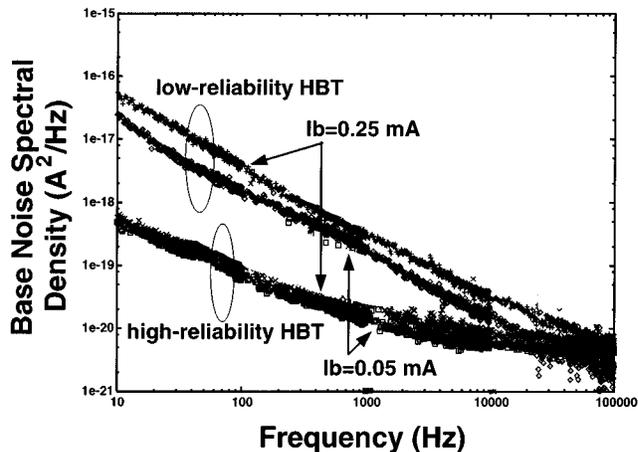
Fig. 6. Base noise spectral density of low and high-reliability HBT's. The bias condition was  $V_{CE} = 3$  V and  $I_B = 50$  and  $250 \mu$ A.
