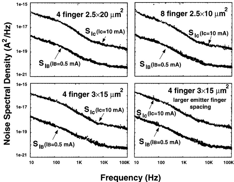
Fig. 4. The base and collector noise spectral density for four different HBT geometry. The periphery/area ratios are indicated in the figure. The tests were performed at  $I_B = 0.5$  mA,  $V_{CE} = 3$  V for base noise and  $I_C = 10$  mA,  $V_{CE} = 3$  V for collector noise. The results permit investigation of periphery/area influence on noise.
