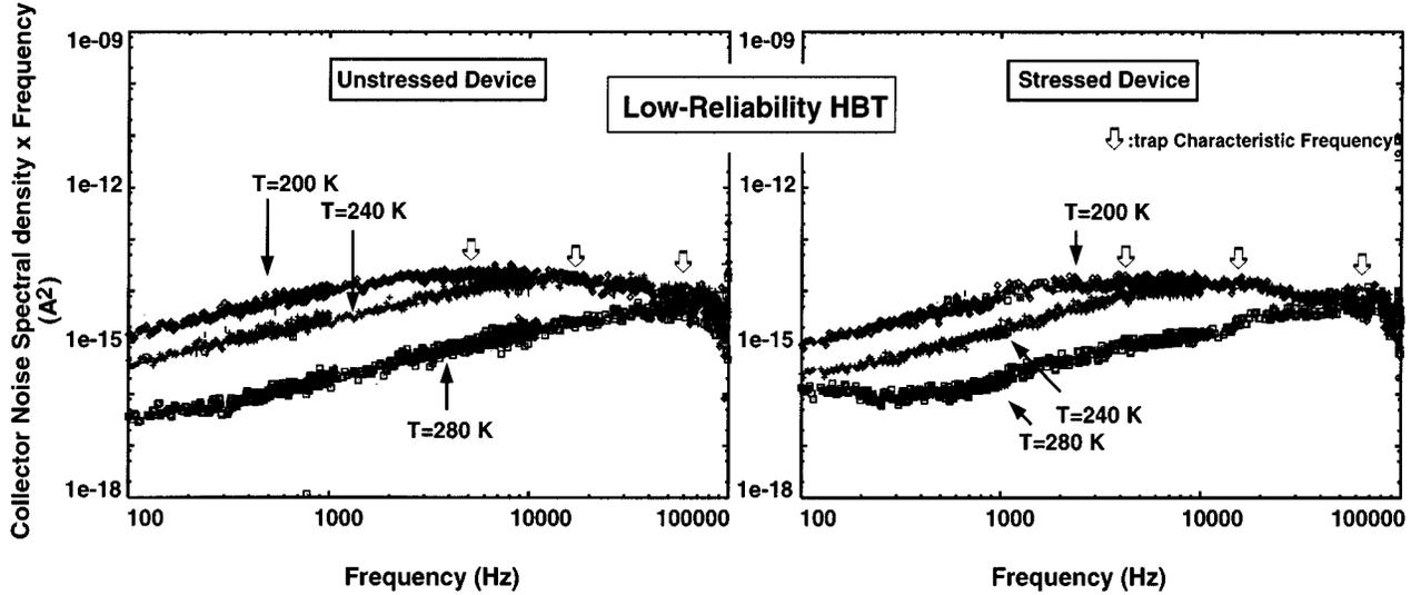
Fig. 9. Temperature dependent collector noise spectral density of unstressed low-reliability HBT. The bias condition was  $V_{CE} = 3$  V and  $I_C = 0.5$  mA.
