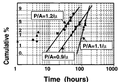
Fig. 3. Results of reliability tests for HBT's with the same emitter area and different periphery/area ratio. The devices were tested at  $J_C = 25$  kA/cm<sup>2</sup> and  $T_j = 125$  °C on medium-reliability wafer.
