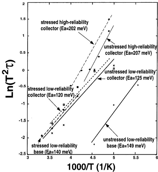
Fig. 10. Arrhenius plots of activation energies of base and collector noise for low and high-reliability HBT's. Results of unstressed and stressed devices are shown.
