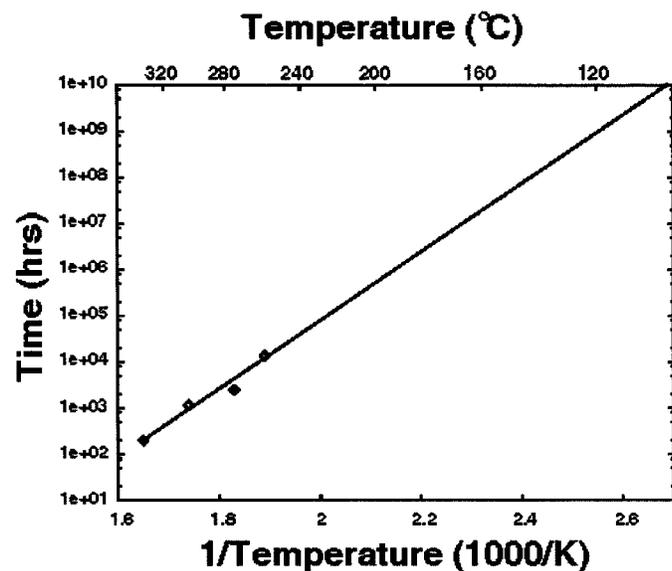
Fig. 2. Estimation of lifetime and activation energy for high-reliability HBT's. The criterion for failure was 30% degradation in the dc current gain. The device was an eight emitter finger  $2.5 \times 20$  μm<sup>2</sup> HBT.
