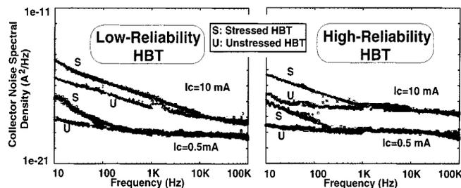
Fig. 7. Effect of stress on collector noise spectral density of low and high-reliability HBT's. The bias condition was  $V_{CE} = 3$  V and  $I_C = 0.5$  and 10 mA.
