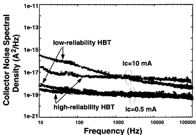
Fig. 5. Collector noise spectral density of low and high-reliability HBT's. The bias condition was  $V_{CE} = 3$  V and  $I_C = 0.5$  and 10 mA.
