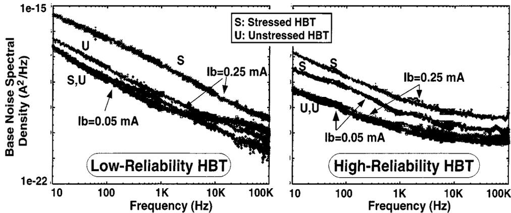
Fig. 8. Effect of stress on base noise spectral density of low and high-reliability HBT's. The bias condition was  $V_{CE} = 3$  V and  $I_B = 50$  and  $250 \mu$  A.
