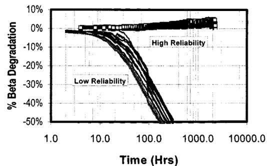
Fig. 1. Variation of dc current gain with time for same HBT's with same geometry on low and high-reliability substrate. The test condition was  $J_C = 25$  kA/cm<sup>2</sup> and  $T_j = 125$  °C.
