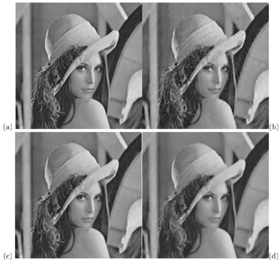
Fig. 10. Image reconstruction results. (a) Reconstructed from both descriptions ( R^* = 0.60 bpp, D_0 = 35.78 dB); (b) MDTC, from a single description, \rho = 0.088 bpp (15%), D_1 = 27.94 dB; (c) MDTC, from a single description, \rho = 0.133 bpp (22%), D_1 = 29.63 dB; (d) MDSQ, from a single description, \rho = 0.090 bpp (15%), D_1 = 28.63 dB.
