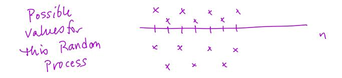
Find mean and autocorrelation and autocovariance Mean:  $M_X(n) \equiv M_n \equiv E(X_n)$ for n odd,  $M_X(n) \equiv \frac{1}{2}(+1) + \frac{1}{2}(-1) = 0$ for n even,  $M_X(n) = \frac{9}{10}(\frac{1}{3}) + \frac{1}{10}(-3) = 0$ SO  $M_X(n) = 0$  for all n
