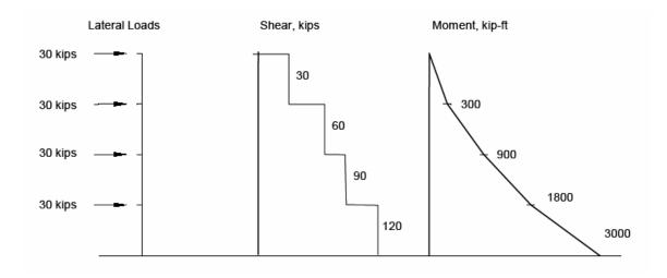
Assume an 8-in. nominal clay masonry wall, grouted solid, with Type S PCL mortar. The total plan length of the wall is 24 ft (288 in.), and its thickness is 7.5 in. Assume an effective depth d of 285 in.
