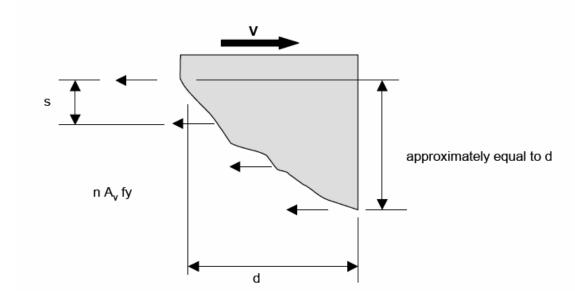
The nominal resistance from reinforcement is taken as the area associated with each set of shear reinforcement, multiplied by the number of sets of shear reinforcement crossing the hypothetical failure surface. Because the hypothetical failure surface is assumed to be inclined at 45 degrees, its projection along the length of the member is approximately equal to d, and number of sets of shear reinforcement crossing the potential failure crack can be approximated as (d/s).
