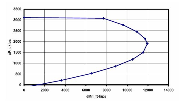
At a factored axial load of 0.9D, or  $0.9 \times 360 \text{ kips} = 324 \text{ kips}$ , the design flexural capacity of this wall is about 4000 ft-kips, and the design is satisfactory for flexure.
