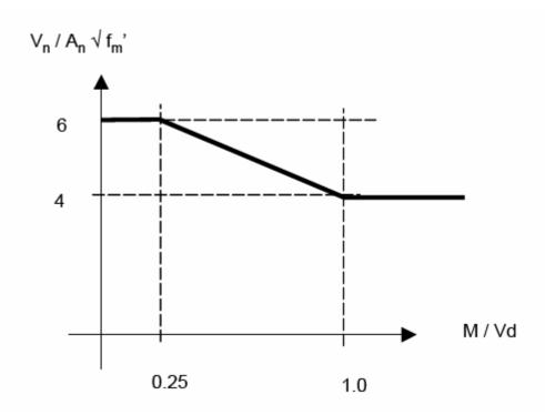
If these upper limits on  $V_n$  are not satisfied, the cross-sectional area of the section must be increased.
