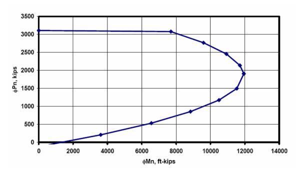
At a factored axial load of 0.9D, or  $0.9 \times 360$  kips = 324 kips, the design flexural capacity of this wall is about 4000 ft-kips, and the design is satisfactory for flexure.
