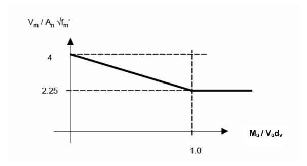
Just as in reinforced concrete design, this model assumes that shear is resisted by reinforcement crossing a hypothetical failure surface oriented at 45 degrees:
