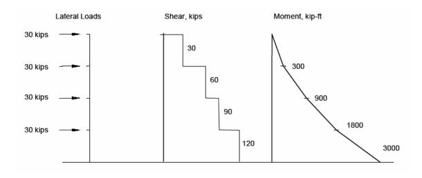
Assume an 8-in. nominal clay masonry wall, grouted solid, with Type S PCL mortar. The total plan length of the wall is 24 ft (288 in.), and its thickness is 7.5 in. Assume an effective depth d of 285 in.
