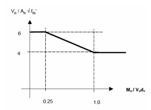
If these upper limits on  $V_n$  are not satisfied, the cross-sectional area of the section must be increased.
