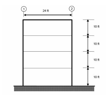
Design the wall. Unfactored in-plane lateral loads at each floor level are due to earthquake, and are shown below, along with the corresponding shear and moment diagrams.
