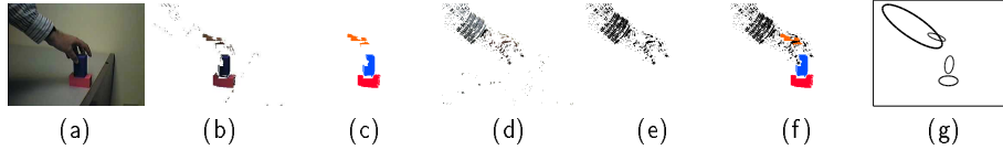
Fig. 2. The processing stages of our tracker. (a) shows an input image. (b) shows the coloured pixels. (c) shows the output of the region grower on (b). (d) shows the moving pixels. (e) shows the output of the region grower on (d). (f) shows the combination of (c) and (e). (g) shows the ellipses that are fit to the regions from (f).
