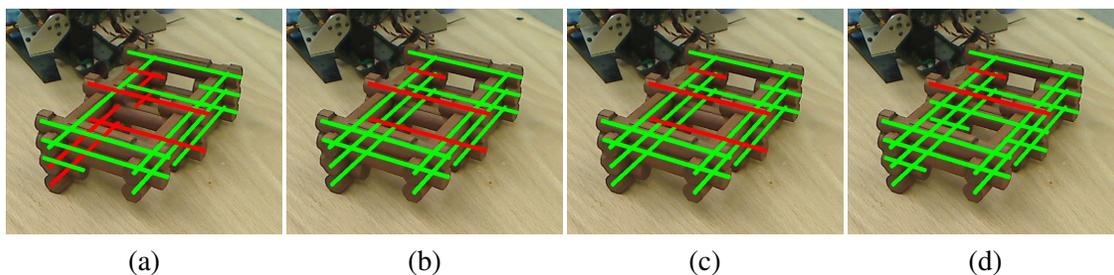
Figure 5. Estimated structure through the following four methods: (a) Baseline structure estimation. (b) Partial disassembly. (c) Multiple views. (d) Combined partial disassembly and multiple views. Overlaid log color indicates correct (green) or incorrect (red) estimation of log occupancies.
